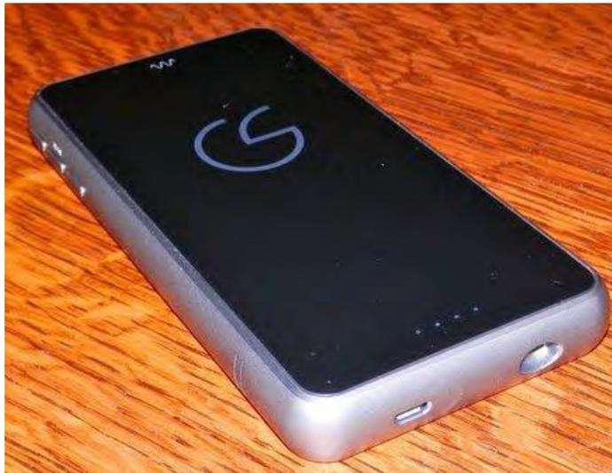
**On the heel of the Companion One we find a USB power port (left) and USB data port (right)**
