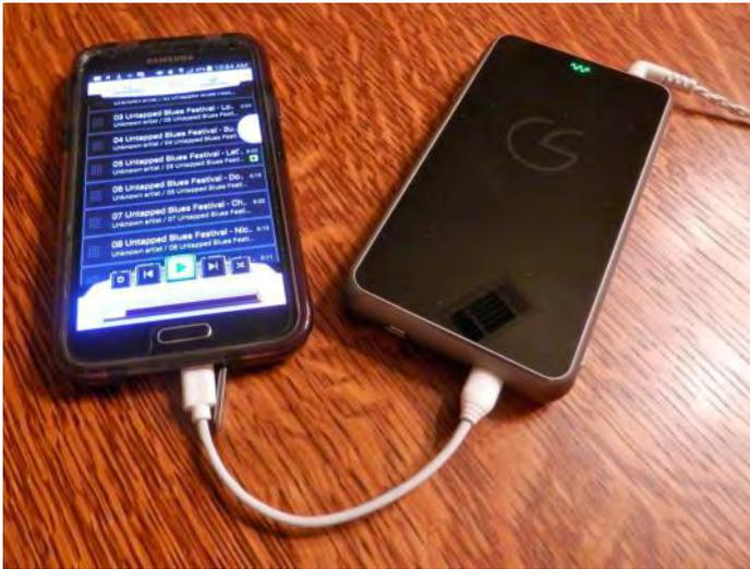
***The Companion One plays digital audio files directly from an Android device (the author's Samsung Galaxy S5), via a Micro USB-to-Micro USB adapter cable.***
