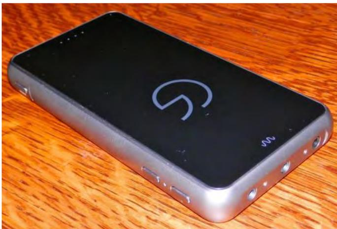
***On the right side of the Companion One (facing the camera in this view) we see the On/Off switch (left, in this view), the Up/Down Volume controls (right, in this view), and the tiny recessed Gain indicator lamp nestled between the Volume buttons.***
