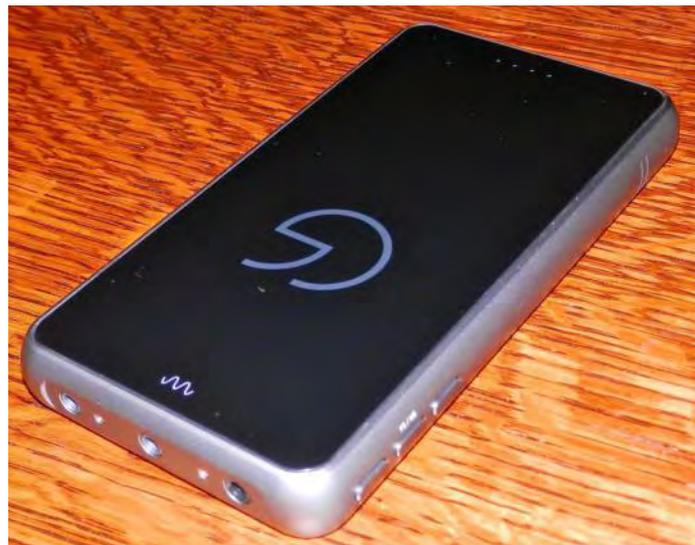
**The top of the Companion One sports a headphone jack (left, in this view), an analogue line-out jack (centre), and coaxial/optical S/PDIF jack (right). On the side of the unit we see the Audio Mode switch (nearest the top), the Connect Mode switch (centre), and High/Low Gain switch (right, in this view).**
